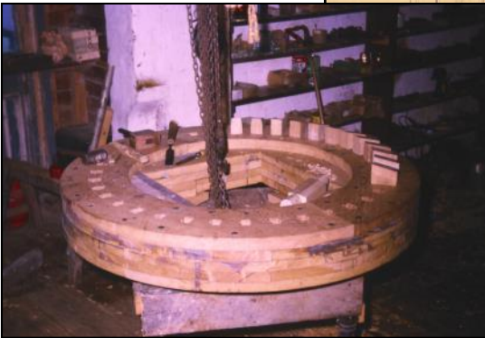
Above: The new brake wheel of the windmill takes shape in Derek Ogden's workshop at Great Alna, Warwickshire.
