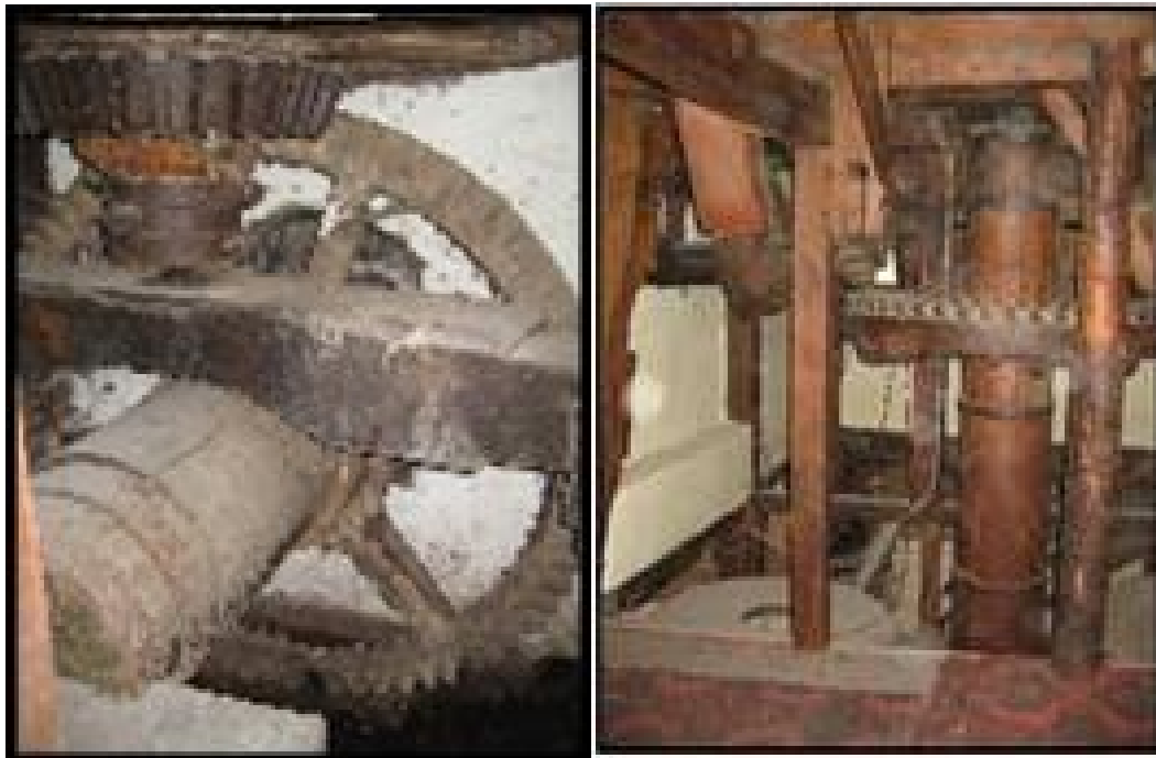
The wheel shaft, pit wheel and wallower of the SE set of gears - The SE set of gears.
