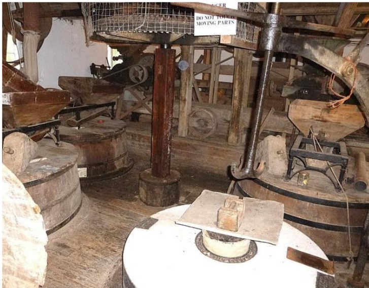
The stone floor: note the stone crane on the right
