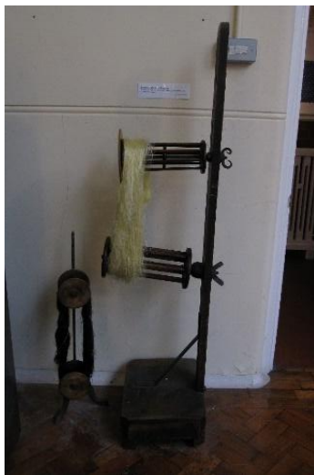
Above, left to right: Spool winder, Cord twister, Tassel former Left: 'Rice' – Wooden device with 2 shaking arms used to prepare hanks of silk for transfer to skeins
