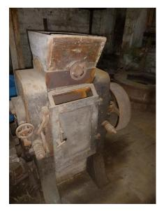
The Daverio roller mill is not one that I have seen in any other mill in the UK and is possibly unique. In April 1879 Henry Simon was advertising 'Daverio's Patent Roller Mill System'. Henry Simon used Daverio three-high roller mills in his first complete all-roller mill plant to operate in England without the use of millstones. This was purchased by McDougall Brothers for their Manchester mill in 1878.
