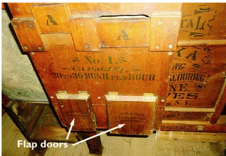
Figure 5: The discharge flap doors and air inlet sliders (marked 'A') on the discharge trunk
