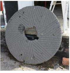
The millstone on the left at Heckington is made from a single piece of French burr. On the right is a grey stone of black lava from Mayen near Cologne, hence the alternative name 'cullen' or blue stone. It is dressed to run anti-clockwise and comes from Dobson Windmill, which is unusual because its sails rotate clockwise.
