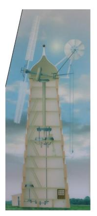
The mill contains a good explanatory diagram (left) but it does highlight just how much ancillary machinery has not survived. The basement contains engine driven gearing which then ascends to a set of stones (right) on the first floor. Note the unusual stones furniture. The roller mill seems to have vanished without trace.
