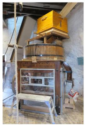
Wholemeal flour is at present being produced on a pair of free-standing Derbyshire gritstones, mounted on a hurst frame by H Onyon of Sleaford, and powered by a Ruston & Hornsby oil engine housed in an adjacent cart shed.
