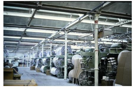
The machines are now all electrically powered so there is no longer any line shafting or belts in position, but the need for good light provided by the large strip lights and the northern light roof is very evident. This was a specially arranged visit to a fully working mill, definitely not a museum, and I have not been able to get inside any large working mills since.
