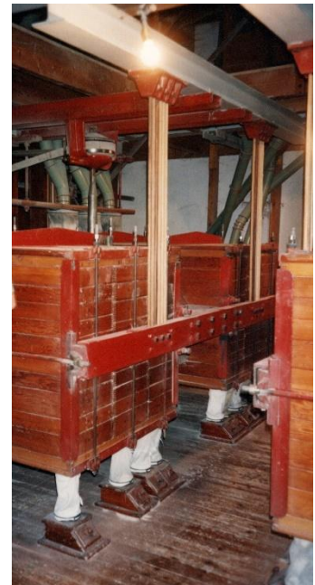
These photos show a spiral seed separator, two of the roller mills, and two of the plansifters.
