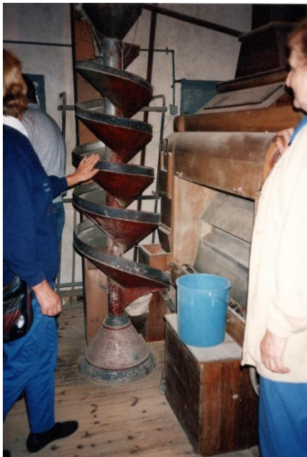
These photos show a spiral seed separator, two of the roller mills, and two of the plansifters.
