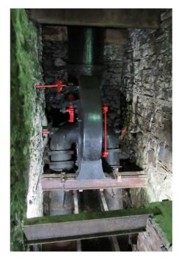
Finally I should mention the Vortex turbine (left) with a fall of 21ft, a suction of 14ft, and a rated power of 20hp (15Kw), supplied by Gilkes of Kendal in 1896, which occupies the original wheelpit.
