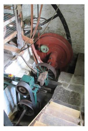
The waterwheel was removed and replaced with a Thomson double-vortex turbine, built by Williamsons (now Gilbert Gilkes & Gordon Ltd) of Kendal. This is thought to be the only remaining working variety of its type. The turbine which generated 10hp (7.46kW) drove a range of woodworking machinery — a rack sawbench, circular saw, planer, and lathes — by a series of belts and pulleys off a central line shaft.
