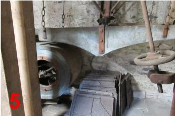
The groats were then transformed into meal in a second pair of stones made of French burr [6]. The cast iron plate on these meal stones reads KAY AND HILTON, FLEET STREET, LIVERPOOL, 1863, and they are also 4ft 6in in diameter.
