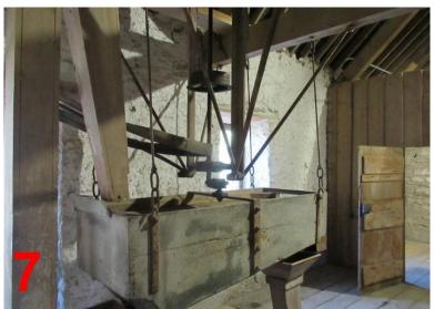
All of the machinery is in its original position complete with connecting belts and chains, apart from the cast iron perforated plates of the kiln, which are stacked below the fanner/winnower [5].
