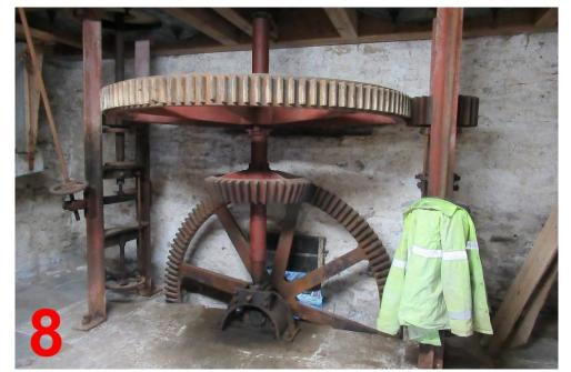
The metalwork was all cast in Strabane in 1862, including the 17ft 6in diameter 5ft 2in wide high breastshot waterwheel, which will soon have 48 new buckets when the next stage of the restoration happens.
