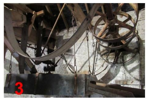
The dried oats were tipped into a small hopper [2] before being transported up the corn elevator and through a corn cleaning sieve, the dark wooden object at the lower left of the picture [3].
