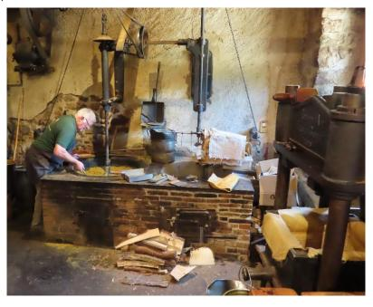
First the seeds are crushed between a small pair of metal rollers, which jammed at first because the 'miller' put too Then they are much in. transferred to a large stone crushing mill with sweeps (above right). When ready, they are carried across to a large frying pan over a pinewood fire (left). The crushed seeds have to be continually stirred by hand and by sweeps to prevent them burning.
