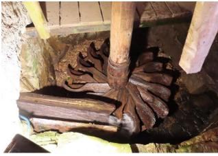
The oil milling machinery is virtually identical to that which we had seen being demonstrated at Moulin des Massons. The crushing mill (*left*) is driven by line-shafting and belts, which also drive the hydraulic pump which operates the press (*right*).
