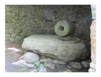
A separate open-fronted stone building further down the slope contains a circular trough and crushing stone for breaking clover pods. The seeds are used as animal feed but also planted: clover is a legume which has root nodules containing nitrogen-fixing bacteria, which add nitrates to the soil and are therefore natural fertilisers. The crushing process generates a lot of dust which is why the mill is situated in an open building.
