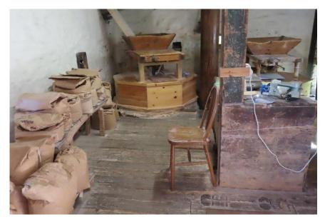
In February 2009 one pair of the original stones (3ft 6in French buhr) turned again to mill wholemeal flour. They now work alongside a second pair of larger French buhr stones which were acquired to replace the older pair of Anglesey stones, which had been used for animal feed and oats.
