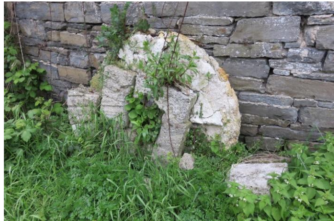
This is what happens to a pair of French buhr stones after they have been left out in the weather for many years.
