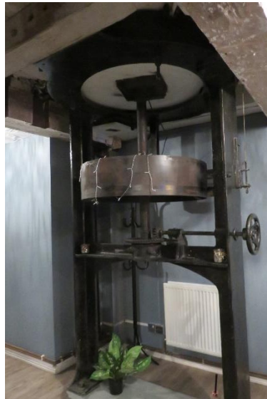
In the Old Mill Restaurant you can still find the metal hurst frames of the millstones which were belt-driven off a turbine and a Ruston diesel engine which is still in its original position.
