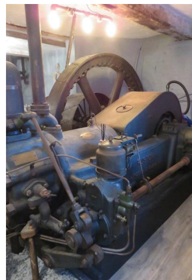
In the Old Mill Restaurant you can still find the metal hurst frames of the millstones which were belt-driven off a turbine and a Ruston diesel engine which is still in its original position.
