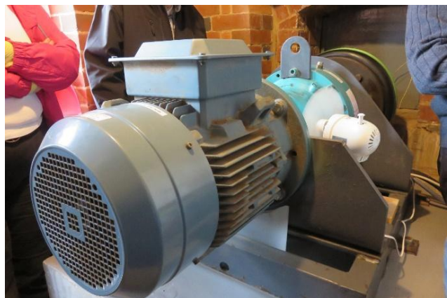
Alternator, gearbox with fan, Fenner-flex rubber coupling – Keith Andrews
