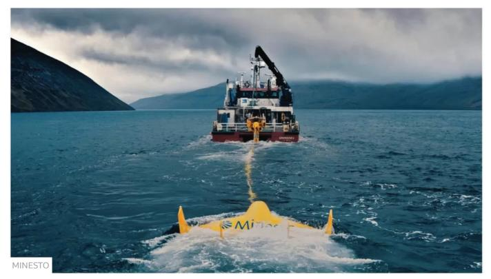
An underwater 'kite' that captures tidal power being towed into place
