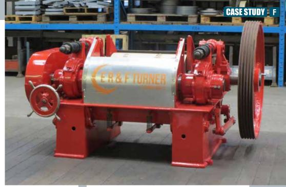
460 is E R & F Turner's latest mills have rolls that spin on a roller bearing, whereas the older machines relied on four Phosphor Bronze Bearing Bushes fitted to the shaft. Out of the four bushes on the vintage model, only one was so badly worn that it needed replacing, the other three were easily restored. A lot of the original guards and castings were also easy to restore, however the logo cover was replaced.
