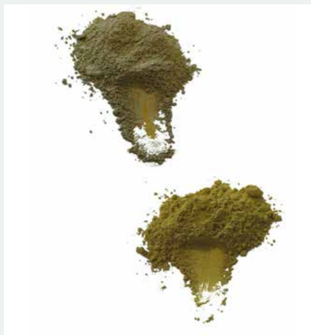
Photo 3: Prevention of yellow spots and streaks in dough Simple quality check: Spreading out a premix containing riboflavin gives an indication of its homogeneity. If the agglomerates are too large, the particles come apart under pressure to form yellow-orange streaks. (left)
