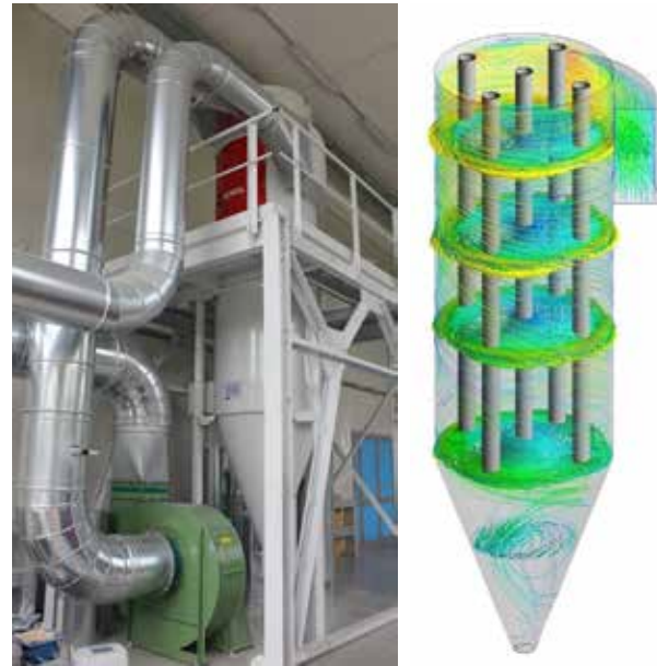
Figure 2: OCRIM Test bed at the University of Parma for the study of fluid dynamics
