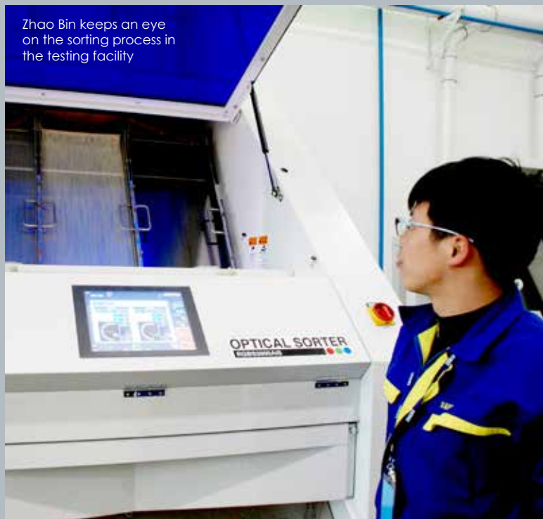
Laboratory equipment for testing rice samples supplied by customers in its laboratory facility on the factory site
