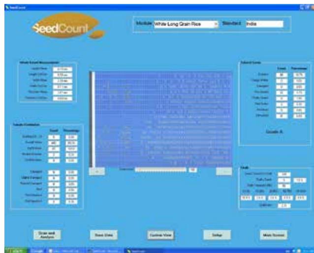
Figure 3: Typical results screen showing the analysis of long grain rice using the Indian Standard.
