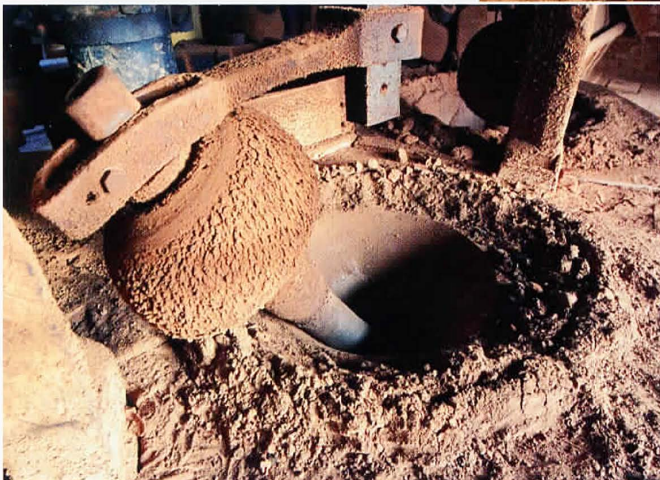
Close view of one of the Grinding mortars at Sharrow Snuff Mill, Sheffield. Photograph - Copyright Jerry Lampson/Wilsons & Co. (Sharrow) Ltd
