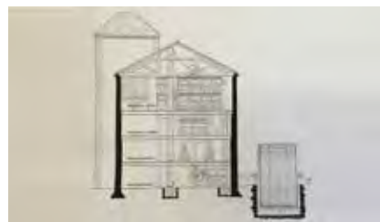
Cross Section of the mill in 1886 showing the 20 foot diameter waterwheel
