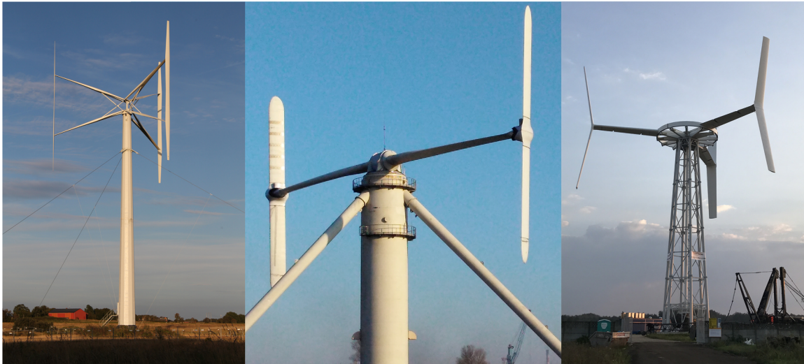
Fig. 5. Left: The 200-kW Vertical Wind H-rotor in Falkenberg. Photo by Erik Möllerström. Center: The 600-kW NENUPHAR onshore prototype. Used with permission from NENUPHAR. Right: The 1.5-MW Anew-B1 turbine during installation in October 2017. Used with permission from the Anew Institute.
