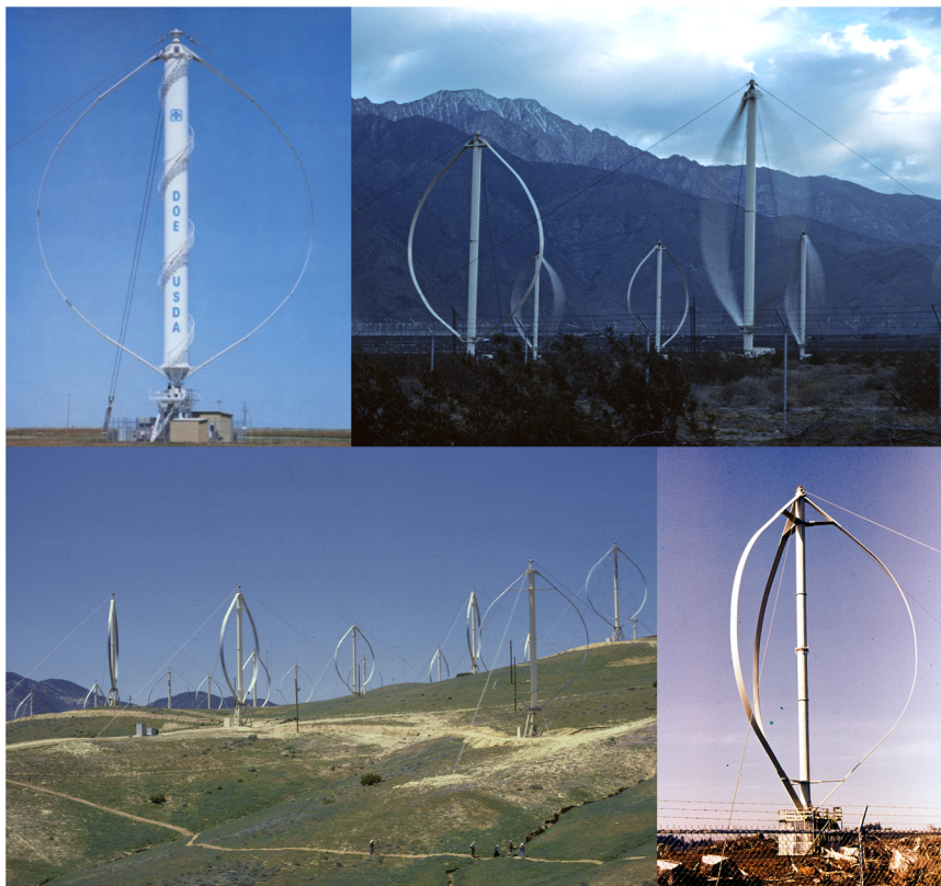
Fig. 1. Upper left: The 34-m 500-kW Sandia research turbine at Bushland, Texas. Photo used with permission from Sandia National Laboratories. Upper right: VAWTPOWER 185 turbines in San Geronio Pass during the 1980s. Lower left: A wind farm with FloWind-19 turbines, in the mid-1980s at Cameron Ridge in the Tehachapi Pass. The 19-m model can be distinguished from the 17-m model by the conventional struts (the FloWind-17 had cable struts). Lower right: The 500-kW ALCOA turbine situated near Newport, Oregon in the 1980s. Photos (except the Sandia turbine) by Paul Gipe. All rights reserved.
