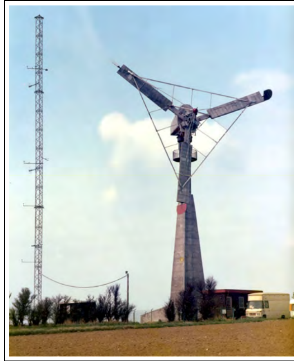
Figure 18. Gedser mill. The grandfather of the Danish design concept. Designed by Johannes Juul, a former student of Poul la Cour, the ungainly but durable machine used struts and stays to brace the rotor as in the F. L. Smidth turbines that preceded it. The turbine is now on display at the Danish Museum of Energy. Note the pitchable blade tips. These were one of Juul's most significant technical innovations and led directly to the success of Danish wind turbines in the 1980s. (The Danish Museum of Energy).
