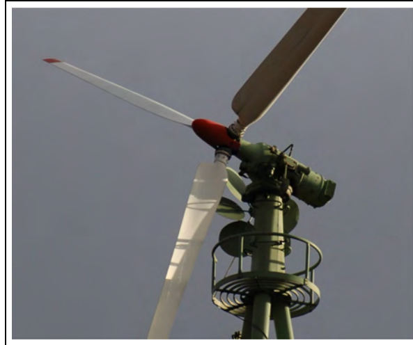
Figure 14. Allgaier. Three-blade downwind 11.3-m (37-foot) rotor with fantail developed by Ulrich Hütter in the early 1950s. Several museum pieces remain, including this one in Holzhausen, Germany. Note the work platform, integrated 10 kW drive train, blades with full-span pitch control, and characteristic Hütter flange at the blade root near the hub. Though it was a downwind turbine, it used a fan tail (the small rotor) to orient the rotor downwind, a feature overlooked by many later engineers. This unit is one of six that was installed by Klöckner-Moeller, a manufacturer of electrical components (2005).
