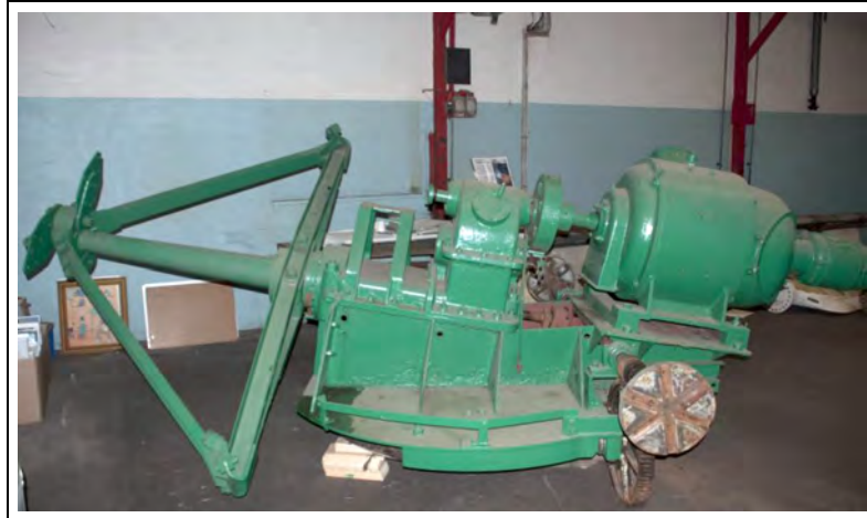
Figure 11. F. L. Smidth Aeromotor drive train. 1941 drive train for a two-blade stayed rotor installed by F. L. Smidth at Ullerslev on the island of Funen, Denmark. The original wooden blades were replaced with metal clad blades in 1954. According to Benny Christensen, board member of the Danish Wind Turbine Historical Collection (Danmarks Vindkraftshistoriske Samling) in Lem, Denmark, this turbine was the last F. L. Smidth in service and operated until 1960. Note the braced rotor, integrated drive train, and fantails (without the blades) for orienting the rotor into the wind.
