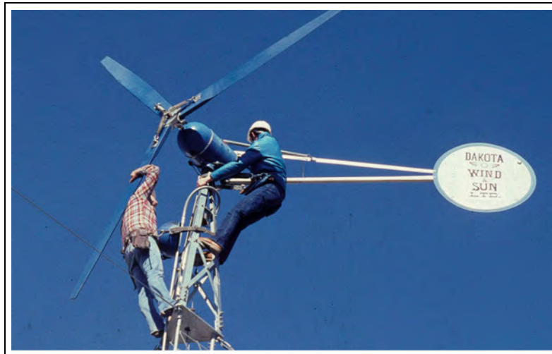
Figure 9. Jacobs Windcharger. The Jacobs design used three wooden airfoils upwind of the tower oriented by a tail vane. Production began in the 1930s and continued into the 1950s. With the revival of interest in wind energy during the 1970s, the rugged Jacobs windcharger was much sought after. Here two technicians replace the brushes on the DC dynamo at West Texas State University's test field in 1979.
