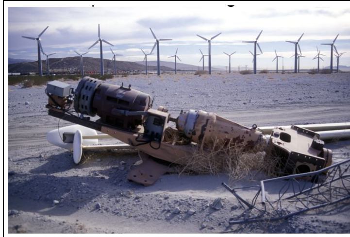
Figure 21. ESI-80. Another US-built series that followed Hütter's design philosophy were the ESI-54 and the later ESI-80 shown here. The ESI turbines also used a downwind, two-blade, teetered rotor driving an induction generator through an integrated gearbox. The brake is mounted on the back-end of the generator (far left). ESI used tip-brakes like those on the Isle of Man turbine, not pitchable-blade tips. The high rotor speed in combination with the downwind design and tip brakes was notoriously noisy. The ESI-80 used a 24-m rotor made up of laminated wood blades coupled to a 250-kW generator. Circa mid to late 1990s.
