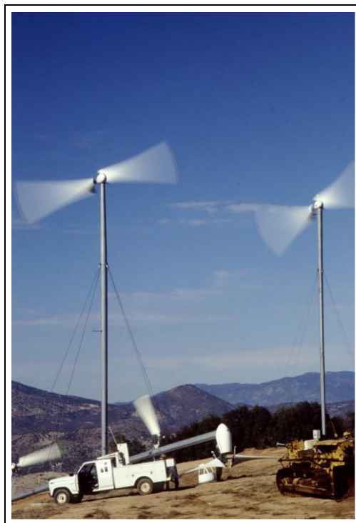
Figure 20. Carter 25. Developed by the father and son team of Jay Carter, Jr. and Jay Carter, Sr., the Carter design grew out of the helicopter industry. The nominally 10-m diameter lightweight, teetered rotor was oriented passively downwind of the tower to drive a 25-kW induction generator. The main spar incorporated a filament winding technology developed for Polaris missile casings. The turbine, created independently of the US wind development program, was introduced in 1979. Downwind two-blade designs such as this generated a characteristic “whop-whop” that annoyed neighbors near Palm Springs, California. Circa 1985.
