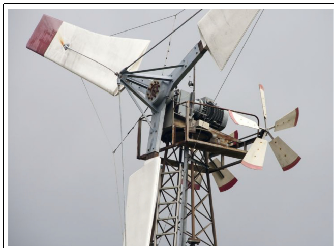
Figure 11. Riisager: One of the pioneering Danish wind turbines during the great wind revival of the 1970s and early 1980s. Laminated wood blades, struts and stays reminiscent of Juul's Gedser mill, and fantails for orientation from the la Cour tradition are all found on this 30 kW version of Christian Riisager's turbine at the Energimuseet , the Danish Museum of Energy near Bjerringbro. Hundreds of derivatives of Riisager's design were installed in California and Denmark. Some were still operating in Californian's Altamont Pass in the mid 2010s.
