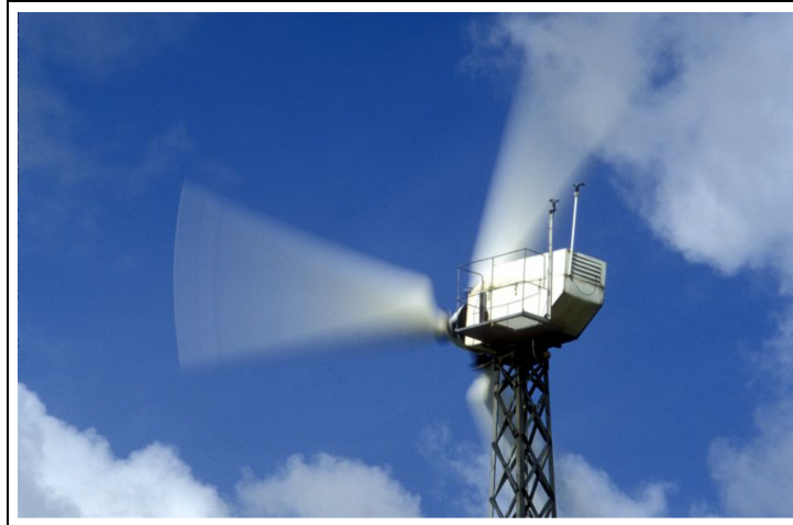
Figure 16. NIVE prototype. Surprisingly durable 10-m diameter turbine built by local “blacksmiths” or machinists from off-the-shelf components in 1978. This 22 kW locally-built wind turbine had been in service for more than three decades before it was removed. Note that unlike the Riisager design, this turbine uses cantilevered blades and an electrically-driven yaw system to point the turbine into the wind. 1998.
