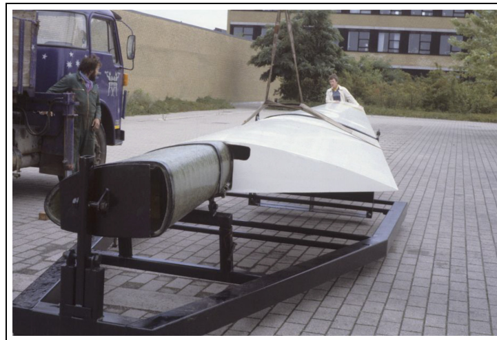
Figure 9. Volund blade. Danish manufacturer Volund built this blade using a filament-wound spar. Filament winding was being used for missile casings in the aerospace industry and was an advanced technology in 1980. However, Volund—and this blade technology—were not successful. Successful blade technology came from a much more prosaic source: the Tvind School. 1980.
