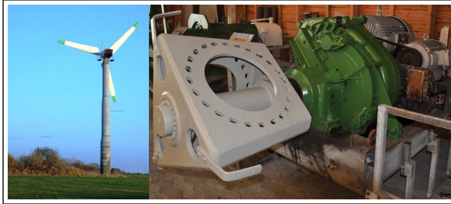
Figure 19. Bonus 55 kW. First Bonus (Danreg Vindkraft) 55 kW wind turbine. Installed in 1981 near the Folkecenter for Renewable Energy in northwest Jutland, the turbine was the forerunner of hundreds of such turbines installed in California in the mid 1980s. Like Vestas' V-15, this Bonus turbine used Økær's 7.5-m (25-ft) blades. In 2004, Bonus was absorbed by Siemens. On the right, Bonus 55 kW drive train. Note the dual generators and large pillow-block main bearing and welded hub. The drive train is part of the Folkecenter for Renewable Energy's collection of historic Danish wind turbines and components. (Preben Maegaard).
