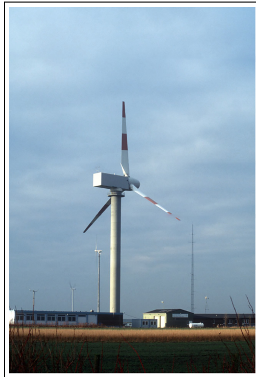
Figure 7. MAN WKA 60. The boxy nacelle on the 60 m (197-ft) diameter upwind turbine looks like a Würst-stand on a stick as one critic called it. Shown here at the Kaiser-Wilhelm-Koog test center in northern Germany, the same site where MAN's ill-fated Growian had been installed earlier. The turbine was not operating when this photo was taken in the late 1990s.
