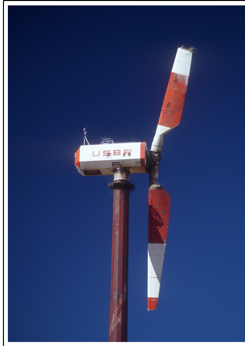
Figure 5. Hamilton Standard WTS-4. One of the most poorly performing large wind turbines developed by aerospace contractors during the 1980s. The WTS-4 had an extremely high specific power of 812 \text{ W/m}^2 and generated only 16 million kWh during its 7000 hours of operation before the teetered, downwind rotor struck the tower in 1994. Late 1990s.
