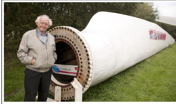
Figure 14. Tvind blade. The late Preben Maegaard, one of the pioneers in the Danish wind revival, stands by the root end of one of the original Tvind blades. The blade is part of Danmarks Vindkraftshistoriske Samling collection of historic Danish wind turbines and components and can be seen at the Folkecenter for Renewable Energy near Hurup, Denmark. The 27-m long blade weighs 5200 kg. Note the blade flange where it mounts to the hub. The flange and the technique for attaching the fiberglass in the blade to the flange were originally developed by Ulrich Hütter in the 1950s and 1960s. Tvind adapted the technique to its pioneering wind turbine in 1975.
