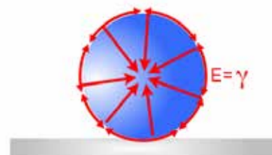
Figure 2. Water on plate forms a sphere due to surface tension
