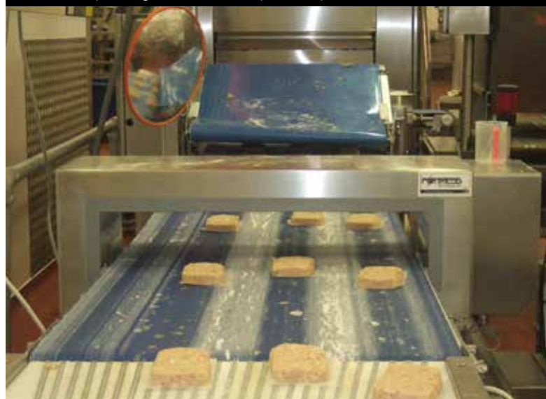
Image 1: Metal detectors tend to be designed around the application, such as incorporating an incline conveyor in this plant
