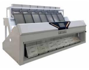
Materials such as white rice, white plastics, white stones all look the same on the surface, for example. Although this is true of our eyes, this is not the case with the NIR sensor, which is able to distinguish between the material differences and can separate these foreign materials out of the product stream. This will significantly improve the safety of the final product.
