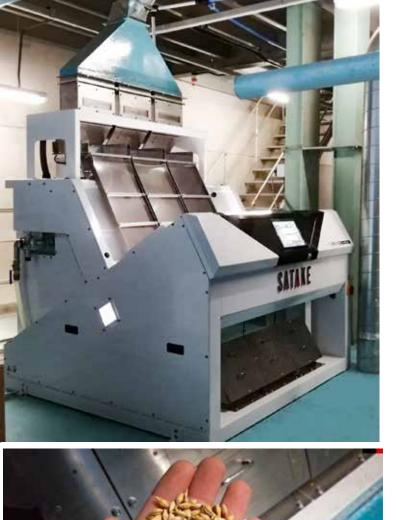
"The Nirami efficiently removes impurities, diseased grains with darkened tips and other defects including immature and brokens."
