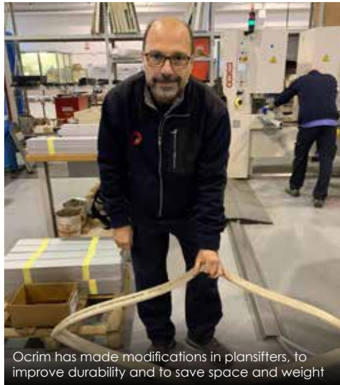
The seals of the new doors for the plansifters are velvet-lined, to ensure they retain their complete seal
