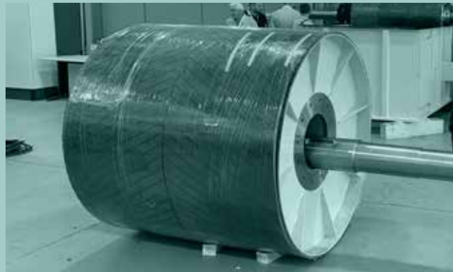
Below: The top and the bottom of it - The massive foot and head rolls of the bucket elevator take shape at Ocrim's engineering plant that will lift grain some 40 metres on a 1.45m-wide belt with seven rows of buckets per metre to achieve 1200 tonnes per hour to be lifted
