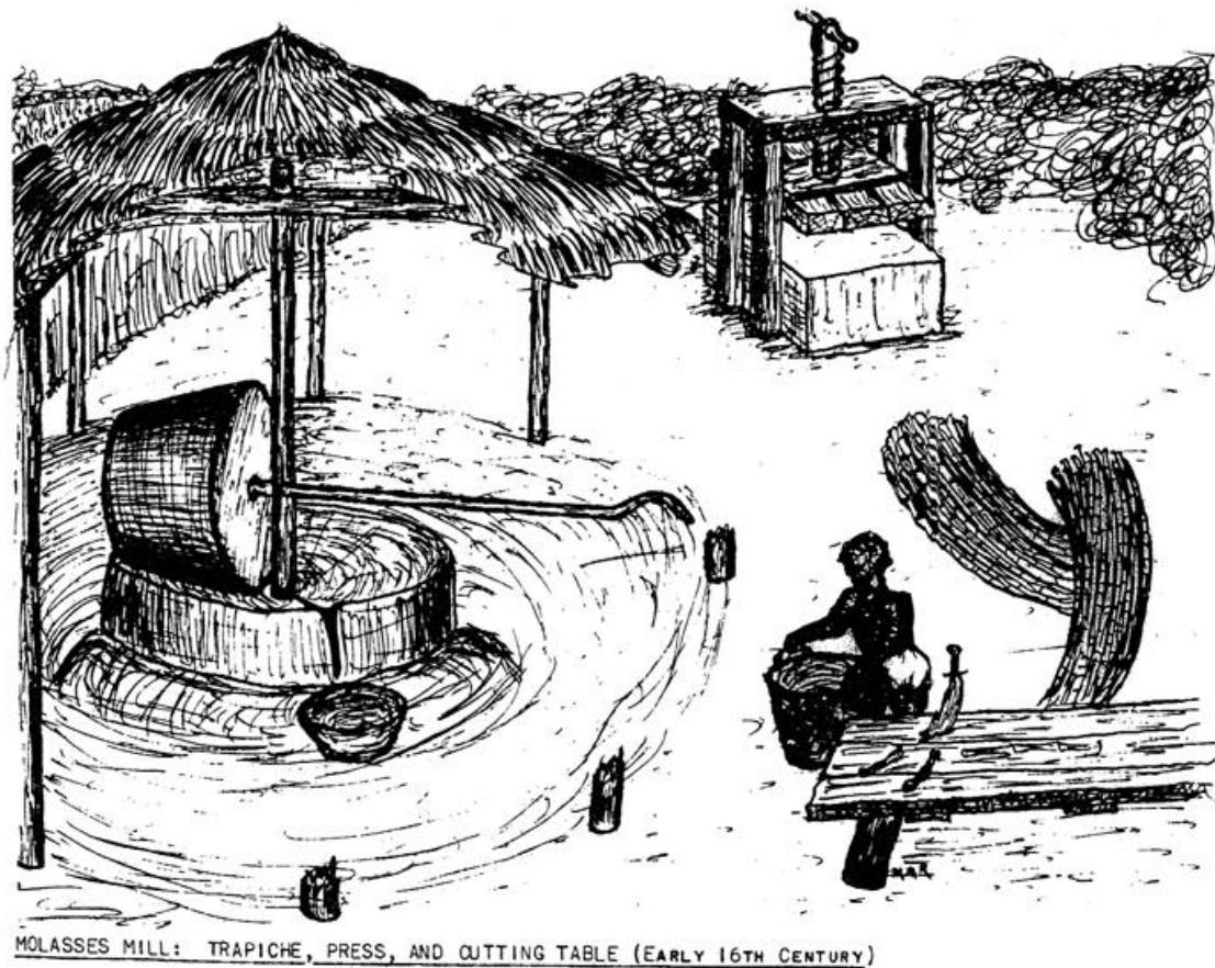
Figure 5. Drawing, included by M. Ratekin in his Master's Thesis of 1952, of a trapiche , shown on the left side of the image, and consisting of a vertical, stone milling-wheel with the truncated-cone shape and activated by animal traction. It swirled on a horizontal stone wheel. To the right rear side a screw press is also shown (Ratekin 1952: 37a). The [burden] animal that pulled the round milling stone would have been tied to the curved end of the horizontal rod coming out from the center of the stone.
