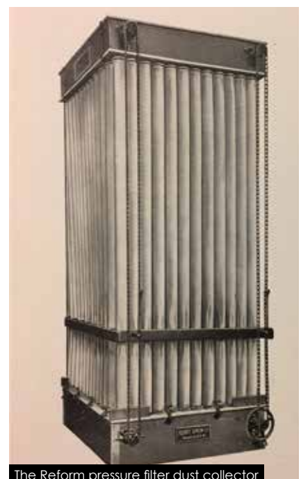
The Reform pressure filter dust collector
