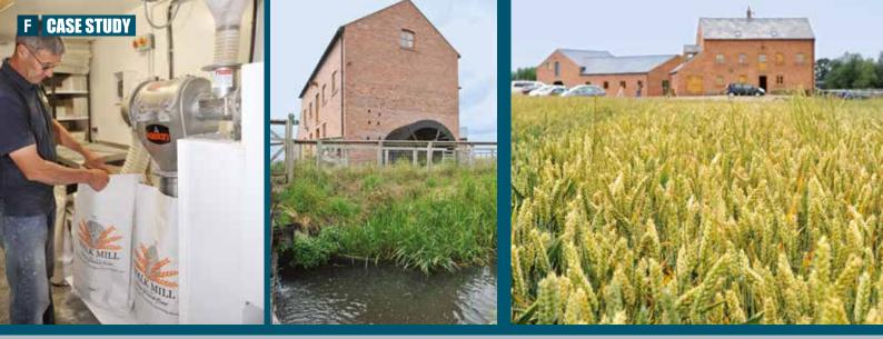
"If the water flow increases, the feeding and milling operations increase at the same rate." Jones adds that a shaft rotation rate of about 40 rpm yields the best quality of flour. The relatively slow, gentle and cool process avoids overheating of the flour, he says, and preserves all the good parts of the grain: protein, oils, vitamins, sugars, starches and bran.
